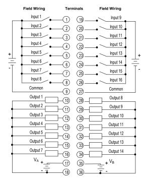
Inputs 1 to 16 form one isolated input group. Outputs 1 to 7 and 8 to 14 form two isolated output groups, each with its own voltage connections. Outputs should be evenly distributed between the two output groups, as discussed under "Output Points versus Temperature".
